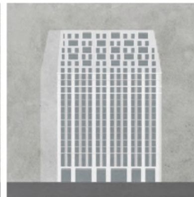
06 Projecting dormers provide articulation to the mansard tier whilst framed surrounds provide articulation to the lower level bays
